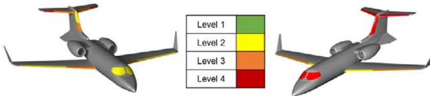
Figure 2. Summary of 1.2 kg. (2.7 lb.) Quadcopter (left) and 1.8 kg. (4.0 lb.) Fixed-Wing (right) UAS Collision Severity Levels on Business Jet Type Aircraft
