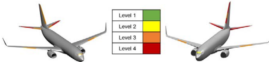
Figure 1. Summary of 1.2 kg. (2.7 lb.) Quadcopter (left) and 1.8 kg. (4.0 lb.) Fixed-Wing (right) UAS Collision Severity Levels on Commercial Transport Jet Type Aircraft
