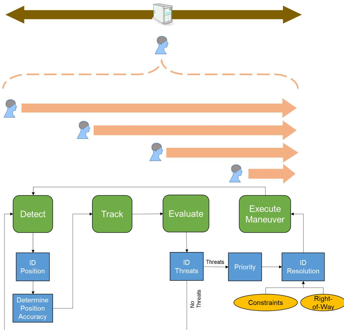
**Figure yy.** Illustration of architectural impacts on human involvement in the system. The flow chart represents the DAA encounter timeline. The brown arrow represents an autonomous system, the orange curly bracket represents a HOTL system, and the orange arrows represent HITL systems.
