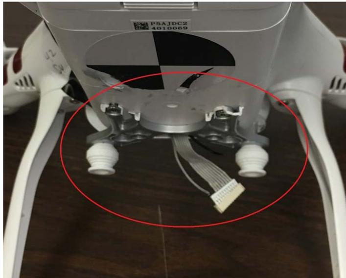
*Figure B - 7 - Complete Payload Separation in Test Article UA17A-22*
