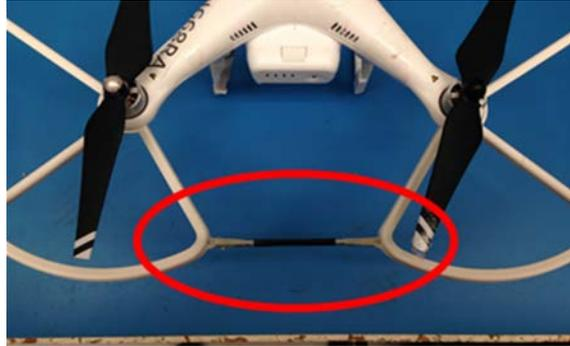
*Figure 13 - Modified blade guard link (highlighted with red oval)*
