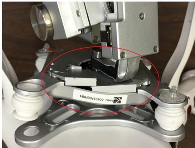
*Figure B - 5 - Damage on Payload Base Plate on Test Article UA17A-11*
