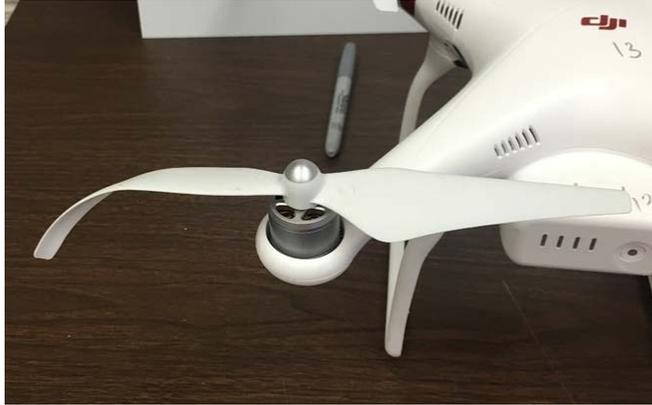
*Figure B - 4 - Bent propeller on the Test Article UA17A-13*
