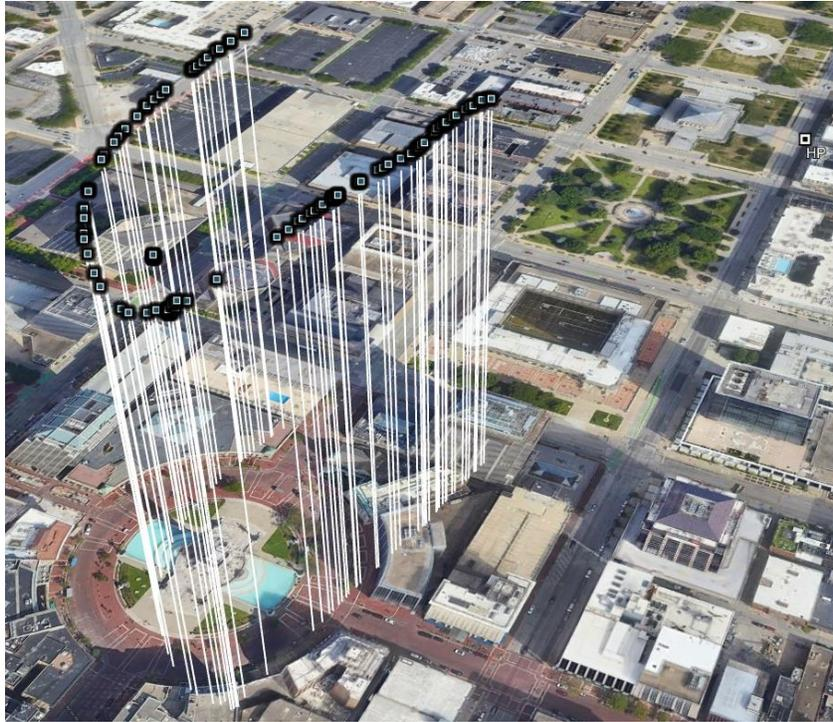
Figure 48. Flight Telemetry of sUAS Collision with Salesforce Tower Building, Indianapolis, IN.
