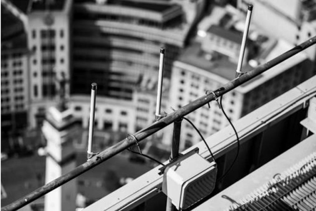
Figure 2. Pierce Aerospace Remote ID Receiver.
