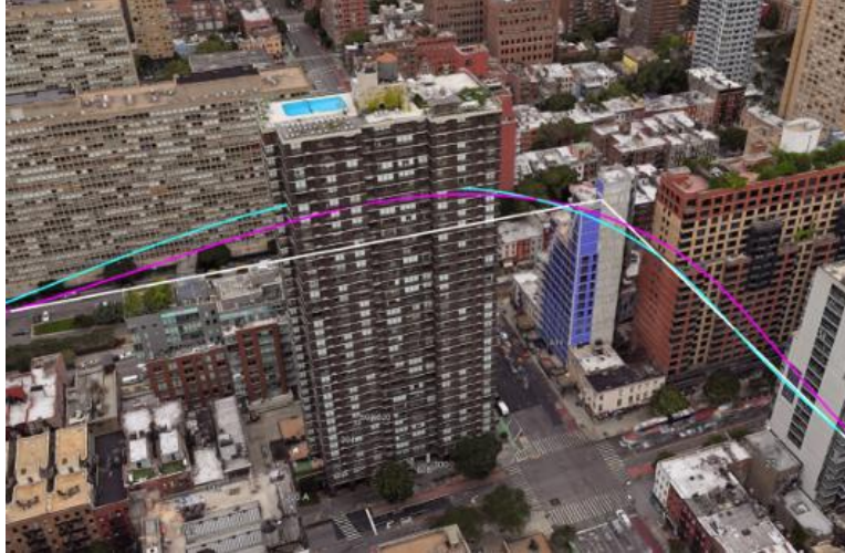
Figure 38. 3D view of the failure of guidance with NY wind in scale of 1.25 (in magenta \rightarrow ) and 1.5 (in blue \rightarrow ) of the wind data in Figure 35 with the fixed-order H_\infty controller and guidance control. This figure is a closer view of the crash area: red rectangle area on the lower left part of Figure 37.
