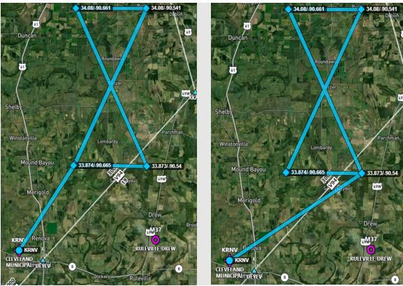
Figure 19. Hourglass flight path for ownship and intruder.
