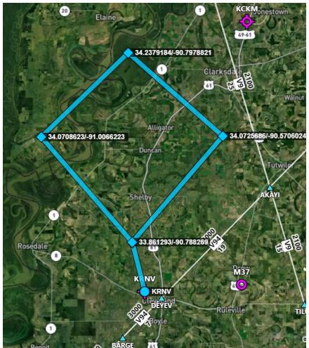
Figure 25. Intruder diamond flight path for overtaking encounters.
